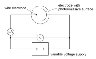
A current is measured on the microammeter only when electromagnetic radiation with a frequency greater than a certain value is incident on the photoemissive surface.
