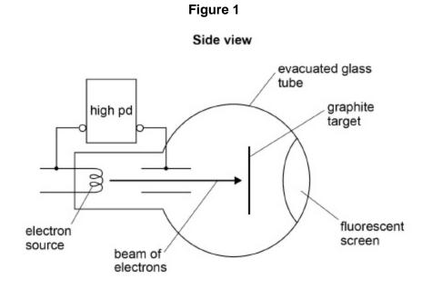
An electron beam is incident on a thin graphite target that behaves like the slits in a diffraction grating experiment. After passing through the graphite target the electrons strike a fluorescent screen.
