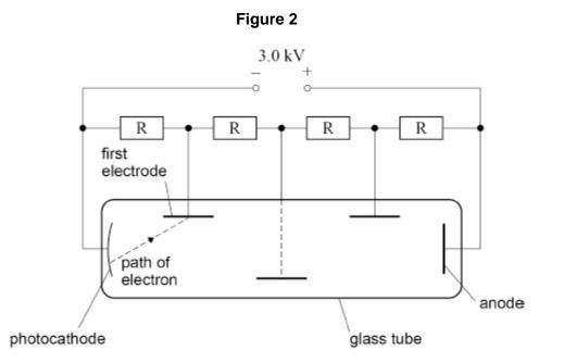
The electrodes, anode and photocathode are connected to a potential divider consisting of four identical resistors R. The emf of the electrical supply is 3.0 kV.
